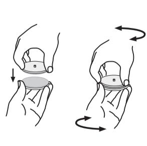
Thoroughly clean the grinding discs, the support angle and the knife before and after each sharpening process. Clean the stones #3000/#6000 by rubbing them lightly against each other in a circular motion.
