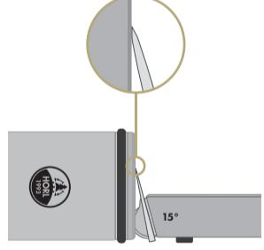
Before using the corundum whetstones, make sure that your knife is ground in on both sides with the HORL Standard Diamond. The cutting edge should burr free.
