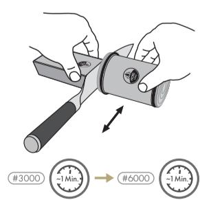
Use the sharpener and the support angle as usual. For the best results, sharpen both sides of the blade for the same length of time.
