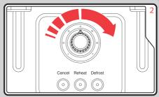
Adjust the Browning Control (2) to the desired setting. Select setting 1 for very light browning from a shorter toasting duration, through to setting 7 for heavier browning over a longer toasting duration.
